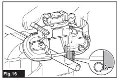
Turn the tool on. Gently lower the blade into the 2. cut. The weight of the tool or slightly pressing the tool will supply adequate pressure for the cutting. Do not force the tool.
