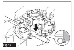
3. As you reach the end of a cut, release pressure and lift the tool slightly so that the tool will not fall against the workpiece.
