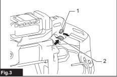
1. Lock-off button 2. Switch trigger
