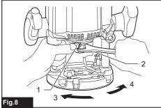
1. Shaft lock 2. Wrench 3. Loosen 4. Tighten
