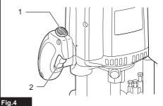
1. Lock button 2. Switch trigger
