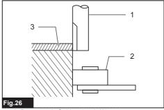
1. Router bit 2. Guide roller 3. Workpiece
