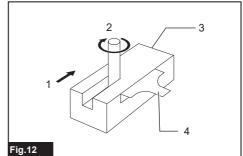
1. Feed direction 2. Bit revolving direction
