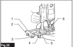
1. Guide holder 2. Fine adjusting screw 3. Clamping screw (D) 4. Clamping screw (C) 5. Guide roller
