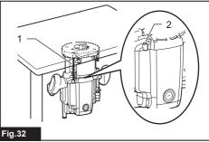
1. Screw M6 x 135 2. Threaded part of the motor bracket
