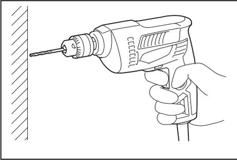
Always hold the tool only by the handle when performing an operation. Do not touch the metal part.
