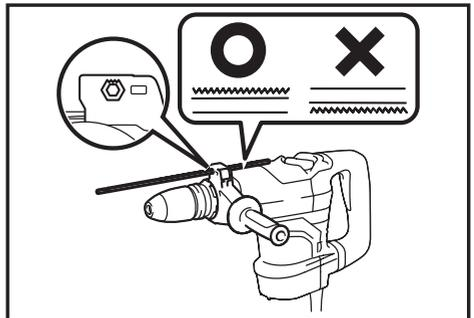
Make sure the toothed side of the depth gauge faces the marking. Adjust the depth gauge by moving it back and forth while pressing the lock button. After adjustment, release the lock button to lock the depth gauge.
