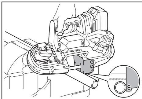
2. Turn the tool on. Gently lower the blade into the cut. The weight of the tool or slightly pressing the tool will supply adequate pressure for the cutting. Do not force the tool.
