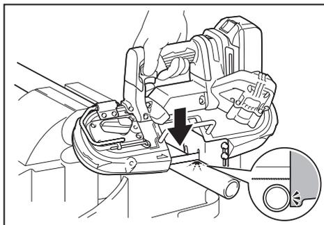
3. As you reach the end of a cut, release pressure and lift the tool slightly so that the tool will not fall against the workpiece.
