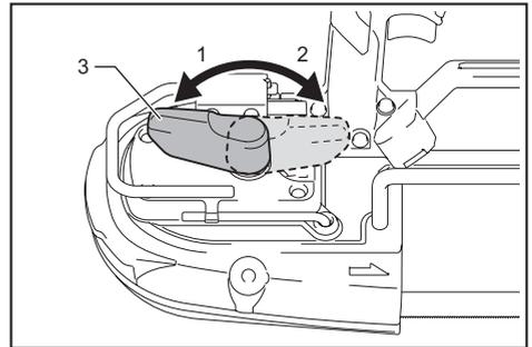
► 1. Tighten 2. Loosen 3. Blade tightening lever
