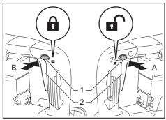
1. Trigger-lock button 2. Switch trigger
