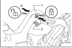
▶ 1. Trigger-lock button 2. Switch trigger
