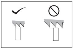
Apply the band saw blade to the suitable cutting position on the workpiece as illustrated.
