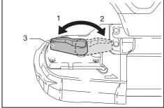
▶ 1. Tighten 2. Loosen 3. Blade tightening lever
