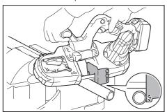
2. Turn the tool on and wait until the band saw blade attains full speed. Gently lower the blade into the cut. The weight of the tool or slightly pressing the tool will supply adequate pressure for the cutting. Do not force the tool.
