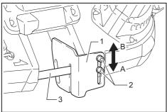
1. Stopper plate 2. Bolts 3. Band saw blade
