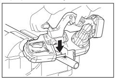
3. As you reach the end of a cut, release pressure and lift it slightly so that it will not fall against the workpiece.
