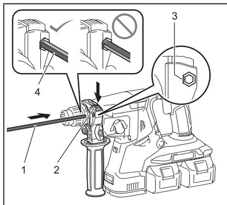
► 1. Depth gauge 2. Lock button 3. Marking
