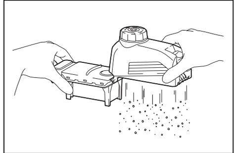
**NOTICE:** When cleaning the filter, do not touch the filter with brush or similar, or blow compressed air on the filter. It may damage the filter.
