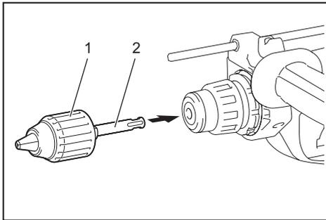
► 1. Keyless drill chuck 2. Chuck adapter
