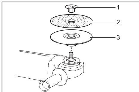
► 1. Sanding lock nut 2. Abrasive disc 3. Rubber pad
