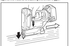
If the head of the pin nail remains above the workpiece surface, drive the pin nail while holding the pin nailer head firmly against the workpiece.
