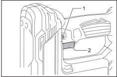
1. Trigger-lock button 2. Switch trigger
