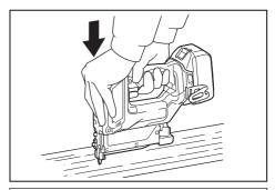
**NOTE:** If the head of the pin nail still remains above the workpiece even you hold the pin nail head, the material may not be suitable for the pin nailer. Continuing to use the pin nailer on such material may result in a damage to the driver of the pin nailer and/ or pin nailer jamming.
