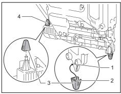
▶ 1. Dent 2. Protrusion 3. Nose adapter 4. Holder
