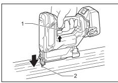
▶ 1. Switch trigger 2. Contact element
