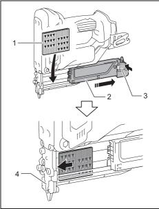
1. Pin nails 2. Magazine 3. Locking lever 4. Driver guide
