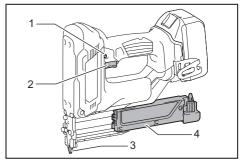
1. Trigger-lock button 2. Switch trigger 3. Contact element 4. Magazine
