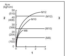
1. Fastening time (second) 2. Fastening torque
