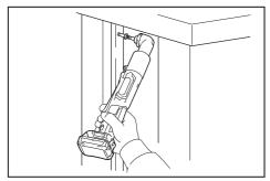
The fastening torque is affected by a wide variety of factors including the following. After fastening, always check the torque with a torque wrench.
