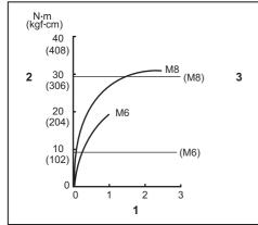
1. Fastening time (second) 2. Fastening torque
