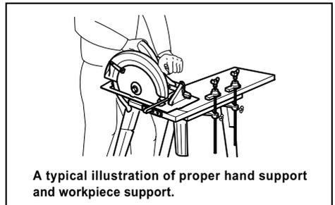
A typical illustration of proper hand support and workpiece support.
