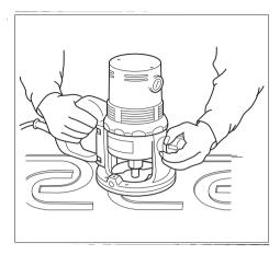
Screw the templet guide on the base plate.
