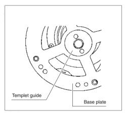
Secure the templet to the workpiece. Place the tool on the templet and move the tool with the templet guide sliding along the side of the templet.
