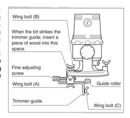
When cutting, move the tool with the guide roller riding the side of the workpiece.
