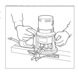
To install the straight guide, insert the guide bar into the hole in the tool base until the notch in the guide bar reaches just under the wing bolt (B). Then tighten the wing bolt (B). Loosen the wing bolt (A) and adjust the distance between the bit and the straight guide. Then tighten the wing bolt (A) to secure the straight guide in place.
