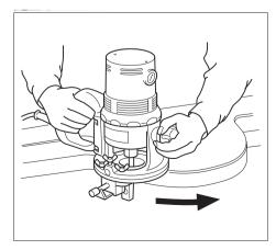
Install the trimmer guide on the tool base with the wing bolts (B). Loosen the wing bolt (A) and adjust the distance between the bit and the trimmer guide by turning the fine adjusting screw (1.5 mm or about 1/16" per turn). At the desired distance, tighten the wing bolt (A) to secure the trimmer guide in place. When adjusting the guide roller up or down, loosen the wing bolt (C), after adjusting it, tighten the wing bolt (C) securely.
