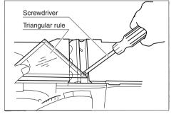
After adjusting both blades, tighten the three installation bolts evenly and alternately with the hex wrench.
