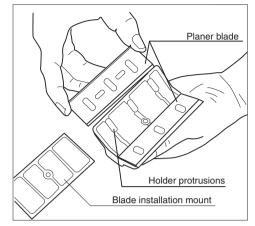
In this condition, hold sharpening holder so that both blades are brought fully into contact with the dressing stone. Thus, both blades will be sharpened simultaneously at the same angle.
