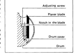
Turn the drum until the blade edge is right in the middle between the front and rear bases.
