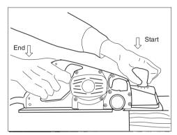
power planer keeps cutting at a speed that will not result in jamming by chips. For rough cutting, the depth of cut can be increased, while for a good finish you should reduce the depth of cut and advance the tool more slowly.
