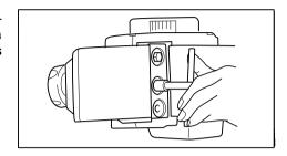
To install the blades, first clean out all chips or foreign matter adhering to the drum or blades. Use blades of the same dimensions and weight, or drum oscillation/ vibration will result, causing poor planing action and, eventually, tool breakdown.
